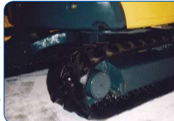
Bridgestone CRT mounted on mini-excavator
