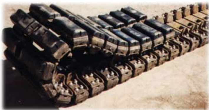
BLS Remanufactured complete track assembly for the Blaw-Knox PF 500 paver
