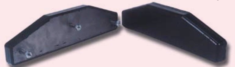
All BLS stabilizer pads are made of a solid block of material, bonded to a steel plate, which then bolts to the machine's outrigger arm.
